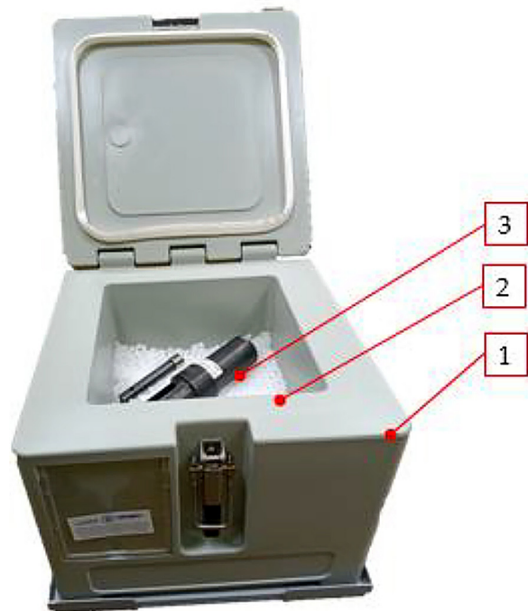
Figure 8. The insulated dry ice storage container and the condition the experimental set-up components, 1 – insulated container, 2 – dry ice, 3 – experimental set-up [17]
