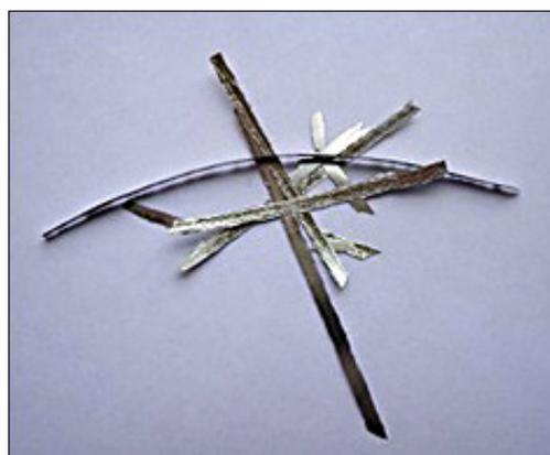
**Fig. 1.** The amorphous  $\text{Co}_{22}\text{Y}_{54}\text{Al}_{24}$  alloy in the form of ribbons
