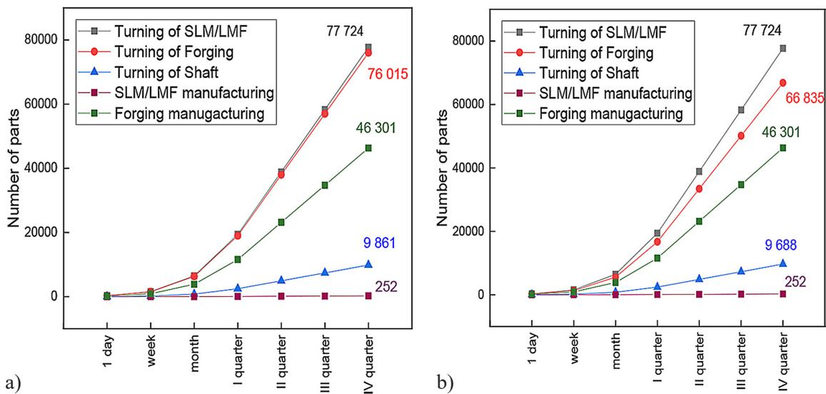
Figure 5. Number of pieces produced during the calendar year during turning and finishing process including machining optimization due to a)  $F_c$  and b)  $R_a$
