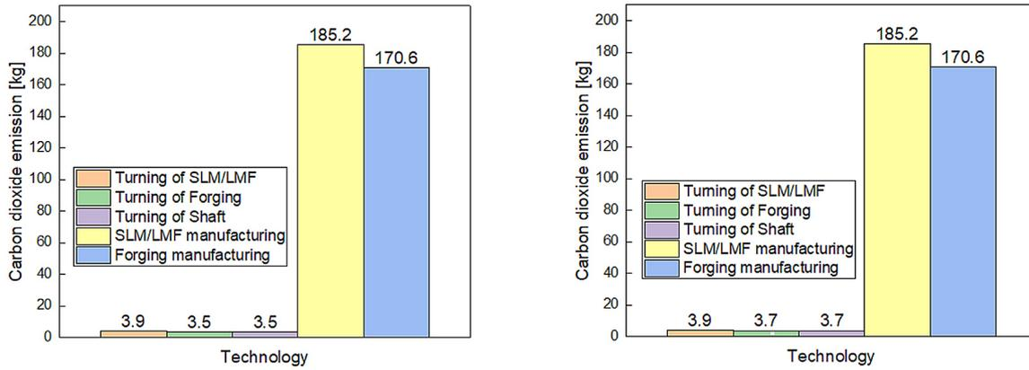
Figure 6. Carbon footprint for one produced cylindrical part by particular manufacturing process including machining optimization due to a)  $F_c$  and b)  $R_a$
