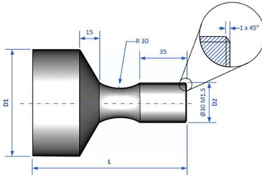
Figure 1. Sample of cylindrical part. Thread at the end (35 mm length)
