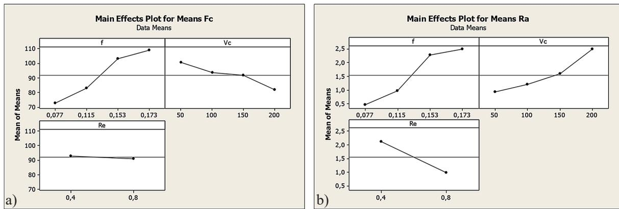
Figure 2. The influence of the cutting data and cutting edge radius on: a) Fc, b) Ra.
