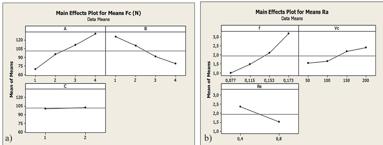
**Figure 3.** The influence of the cutting data and cutting edge radius on: a)  $F_c$ , b) Ra
