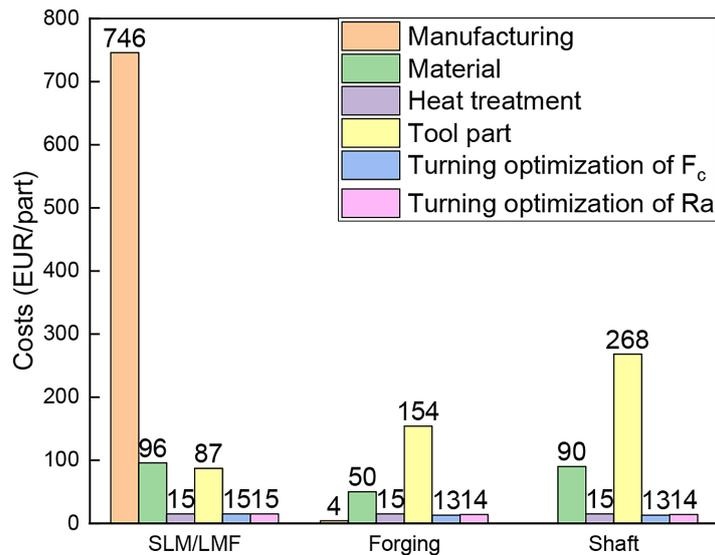
Figure 4. Comparison of costs for individual manufacturing techniques including machining optimization due to  $F_c$  and  $R_a$
