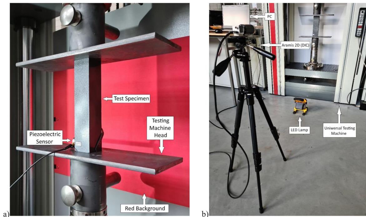
Fig. 3. Experimental test stand: a) experimental test heads with specimen, b) general view of the test stand - Zwick Z100 testing machine with Aramis 2D system
