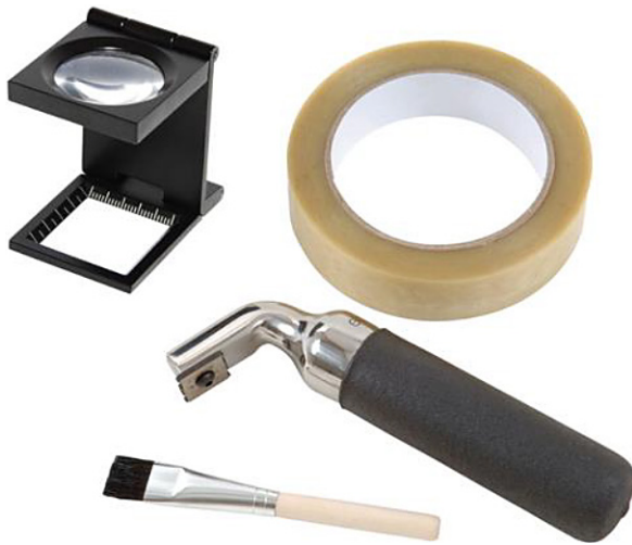
Fig. 4. Toolkit for grid adhesion testing
