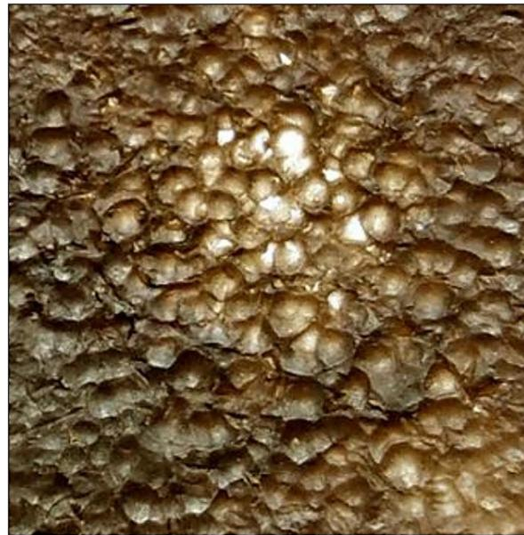
**Fig. 7.** Photograph of the surface of the sample with model pollution after treatment with a pulsating jet of liquid with metal balls, angle 90° (scale 1:8)
