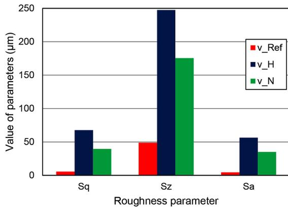
**Figure 5.** Comparison of selected roughness parameters of fatigue fractures of joints of all considered variants for the first measurement area
