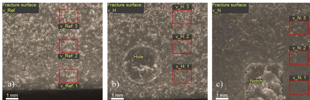
**Figure 4.** Macroscopic views of selected fatigue fractures with marking of roughness measurement areas for the following variants of samples: reference (a), with holes (b) and with notches (c)
