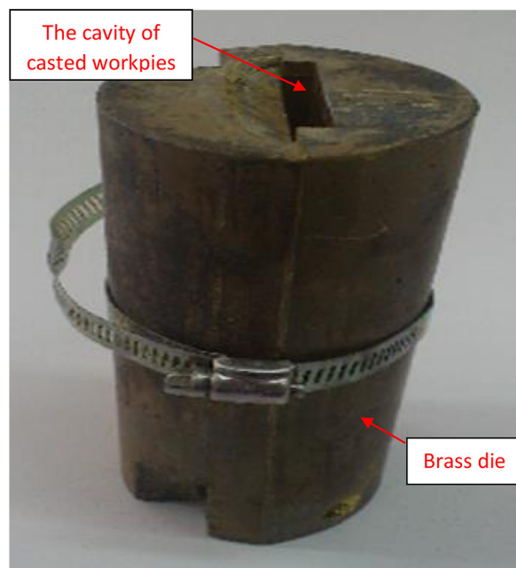
Fig. 2. Brass casting die of a cavity of (160×45×5 mm)
