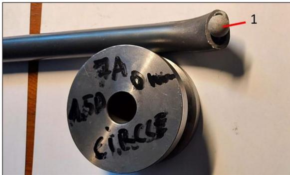
Fig. 22. Ovalization test conducted with a check ball on 16Mo3 steel tubes bent using a circular impression, (1) check ball with a diameter of  $0.86D_w = 13.7$  mm
