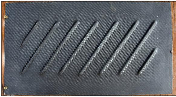
**Fig. 12.** Composite panel reinforced with “shaped” stiffeners
