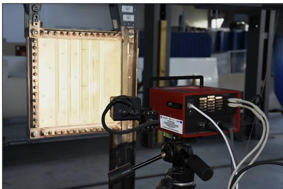
Fig. 5. One of the examined elements together with the Atos 3D scanner
