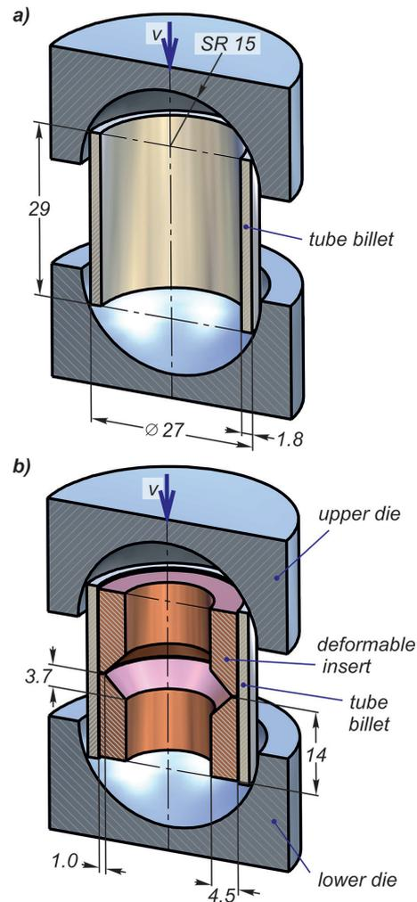
Fig. 1. Schematic of the forging process of a hollow ball with a diameter of  $\varnothing 30$  mm using only two dies (a) and using a suitably shaped deformable insert as an additional tool (b)
