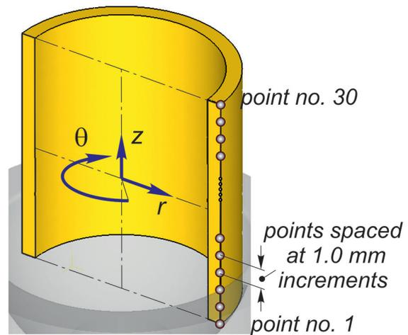
Fig. 7. Arrangement of the 30 tracking points (sensors) on the lateral surface of the billet and the cylindrical coordinate system  $\{r, z, \theta\}$  taken at mid-height of the billet
