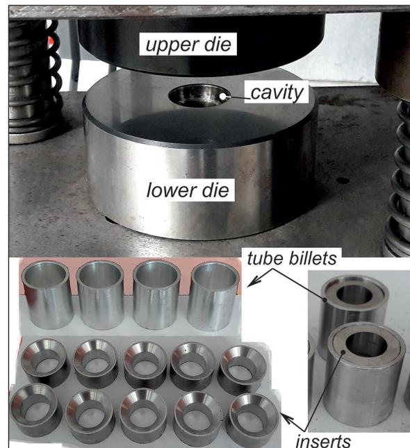
Fig. 4. Photograph of the tools used in the experimental verification and the shape of the samples (the billet from which the ball is obtained and the rings from which the deformable insert is created)
