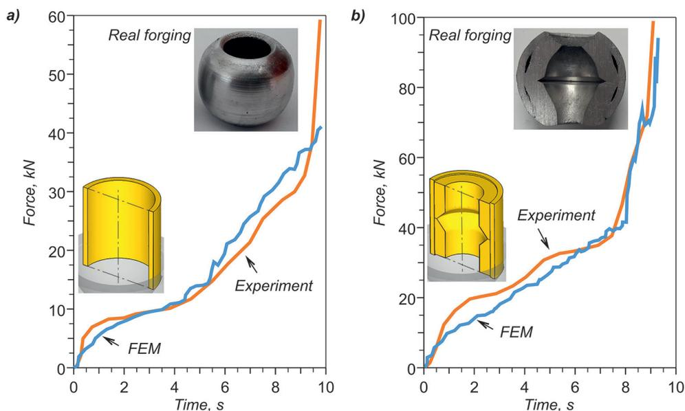
Fig. 5. Shape progression of forged ball forgings without deformable insert (a) and with insert (b) – description in the text
