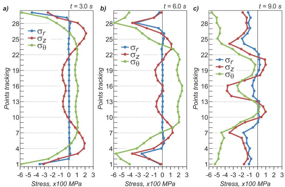
Fig. 10. Distribution of stress components in the sensors (according to Figure 7) for three selected moments of the hollow sphere forging process using a deformable insert
