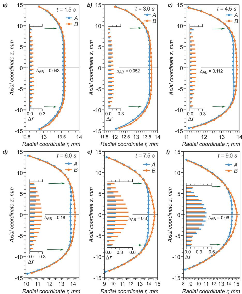
**Fig. 8.** Comparison of the change in sensor coordinates representing the external outline of a forged ball wall without (line A) and with (line B) a deformable insert – full description in the text
