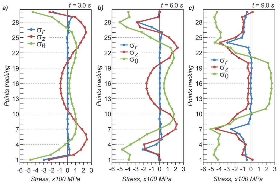
Fig. 9. Distribution of stress components in the sensors (according to Figure 7) for three selected moments of the hollow ball forging process without the use of a deformable insert
