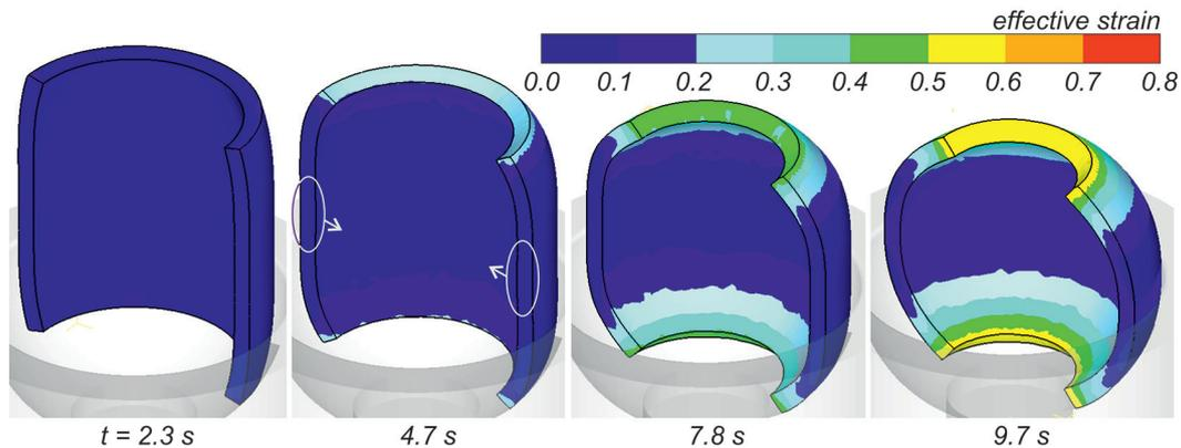
Fig. 2. Shape progression and effective strain distribution during the forging of a hollow ball without a deformable insert – the second figure shows where the concavity of the workpiece wall is being formed
