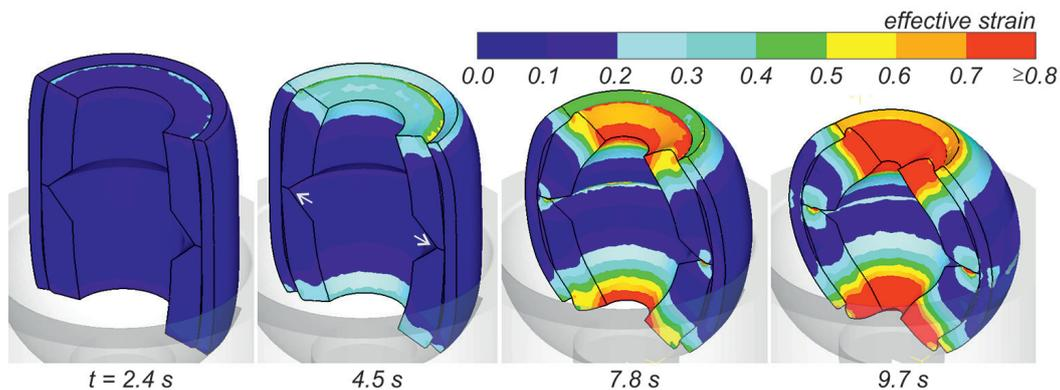
Fig. 3. Shape progression and effective strain distribution during the forging of a hollow ball using a deformable insert (description in the text)
