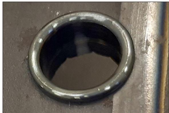
**Fig 2.** Collar and bushing of friction drilled hole
