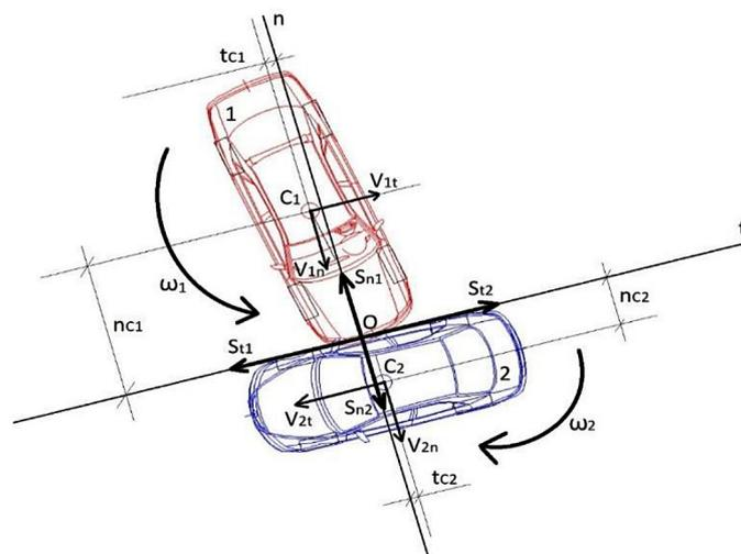
Figure 6. Velocity components and the angular velocities at the start of the collision
