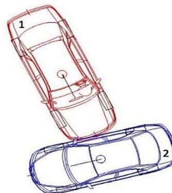
**Figure 3.** The initial location of both vehicles at the beginning of a collision – preparation for determining the necessary angles (Source: PC-Crash)
