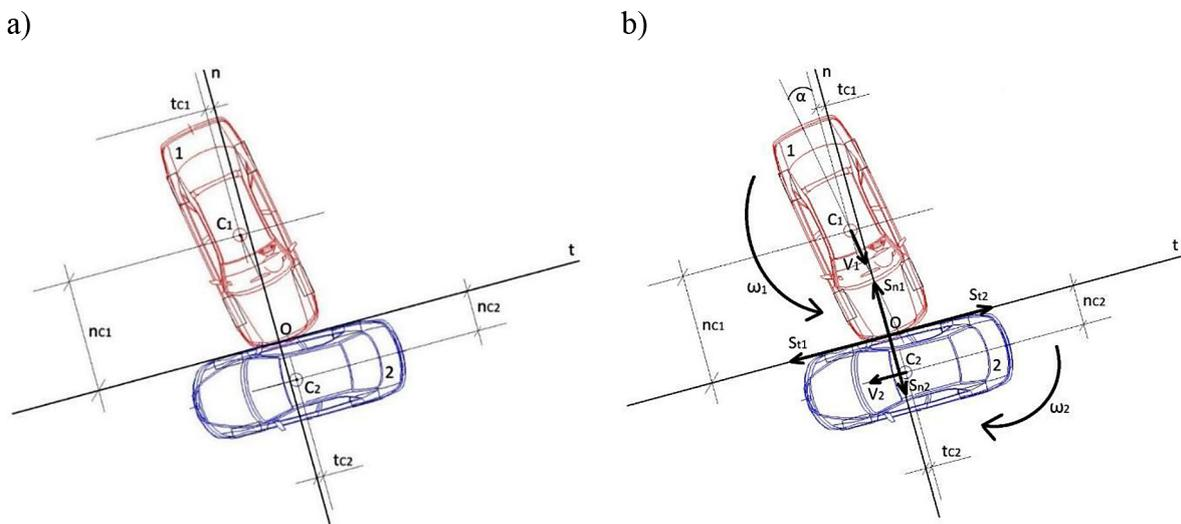
**Figure 5.** a) Location of the center of mass of each vehicle from  $O$  at the beginning of a collision, b) The directions of rotation on a road plane during the collision Source: PC-Crash
