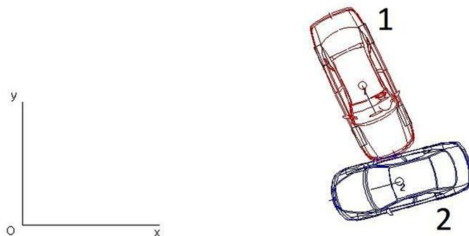
Figure 2. The initial contact of both vehicles at the beginning of the collision (Source: PC-Crash)
