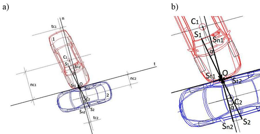
Figure 7. a) The components of the impulses of collision force, b) Magnification of the selected area of Fig. 7a
