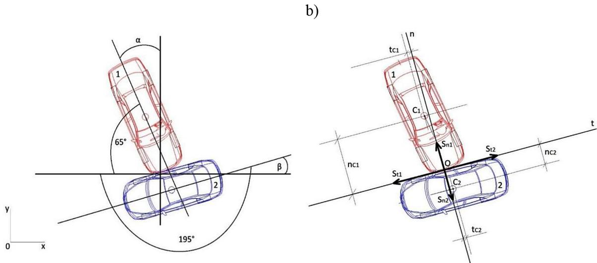
**Figure 4.** a) Mutual location of the vehicle 1 and 2 at the initial moment of the collision, b) The coordinate system  $Ont$  for the side impact collision Source: PC-Crash.
