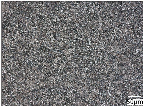
**Fig. 3.** Hardox 600 steel tempered martensite micro-structure. Magn. 500×; etched with 3% HNO<sub>3</sub> (Mi1Fe)
