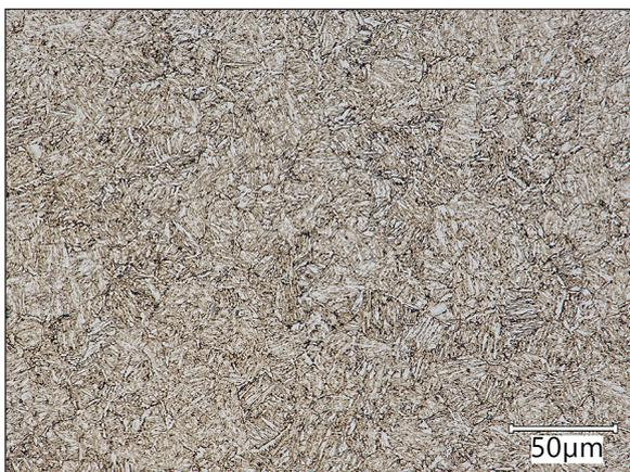
**Fig. 1.** Microstructure of 38 GSA steel. Tempered martensite with bainite. Magn. 500×; etched with 3%  $\text{HNO}_3$  ( $\text{MnFe}$ ), light microscopy
