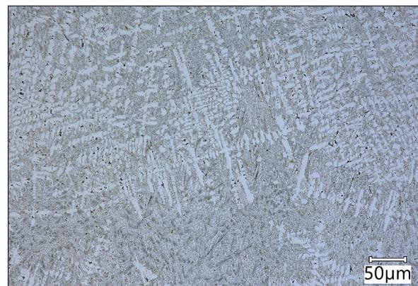
**Fig. 2.** External surface of the EstelMn60 padding weld. Dendritic precipitates of alloy ferrite (light areas) and dark areas of the eutectic system. Magn. 200×; electrolytically etched with chromic acid
