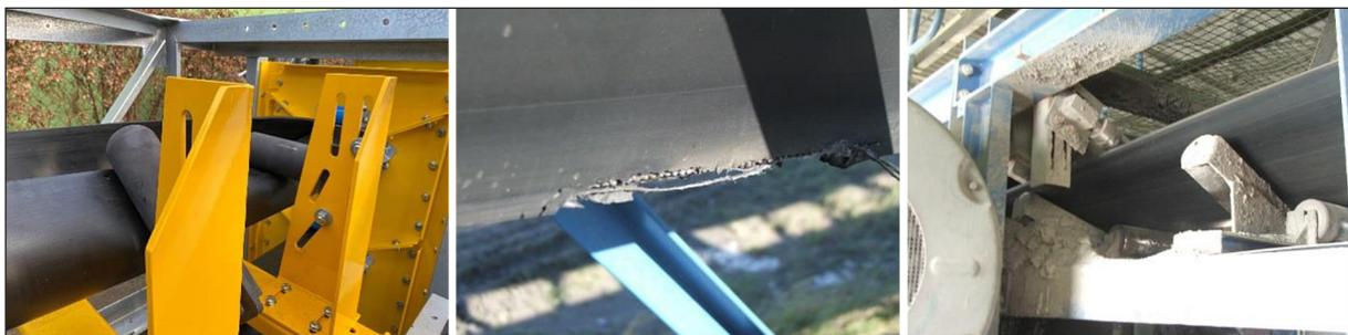
Figure 4. Example of an insufficient contact force on forming rollers
