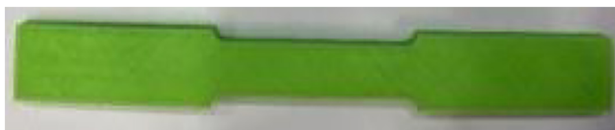
Figure 20. A severely warped PLA dog bone [108]
