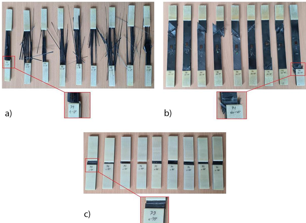
Figure 9. Damaged specimens for material testing: (a) specimens P1÷P9 t-0°, (b) specimens P1÷P9 shr-45°, (c) specimens P1÷P9 c-90°
