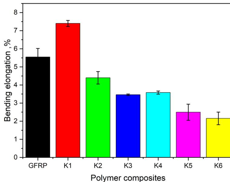
Fig. 7. Comparison of the bending elongation for HFRP (K1-K6) composites and GFRP composite.
