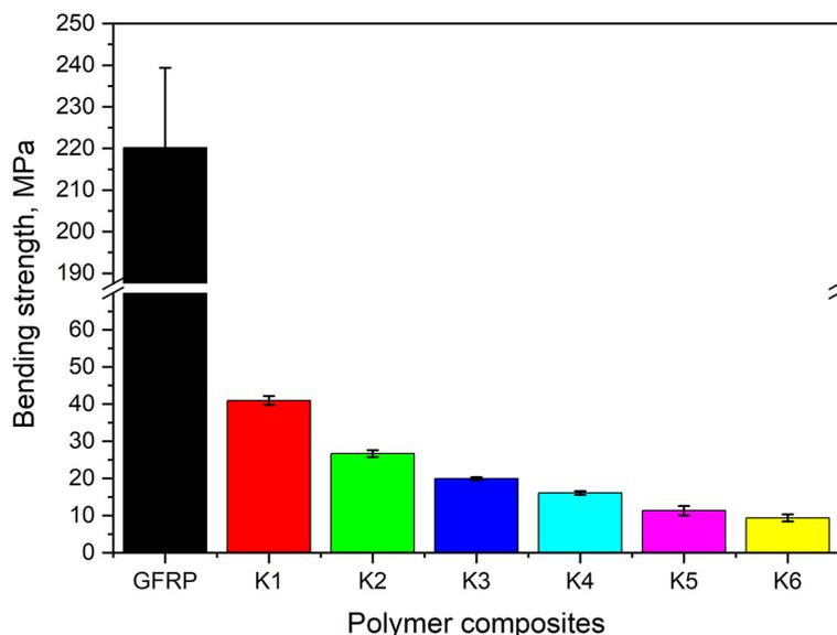
**Fig. 9.** Comparison of the bending strength for HFRP (K1-K6) composites and GFRP composite.
