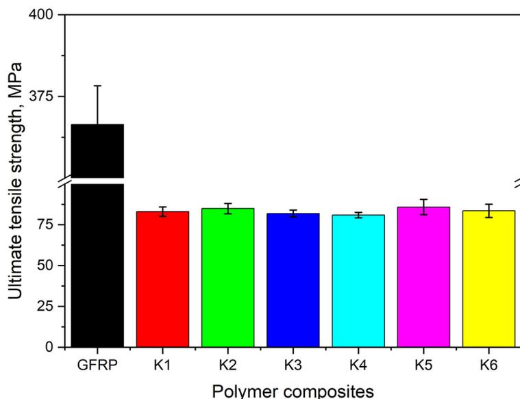
Fig. 5. Comparison of the ultimate tensile strength of HFRP (K1-K6) and GFRP composites.
