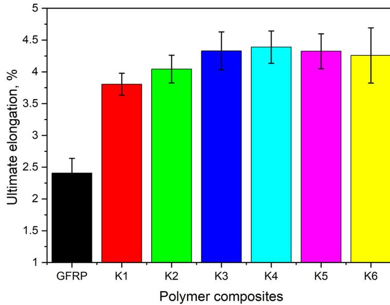
Fig. 4. Comparison of ultimate elongation of HFRP (K1-K6) and GFRP composites.
