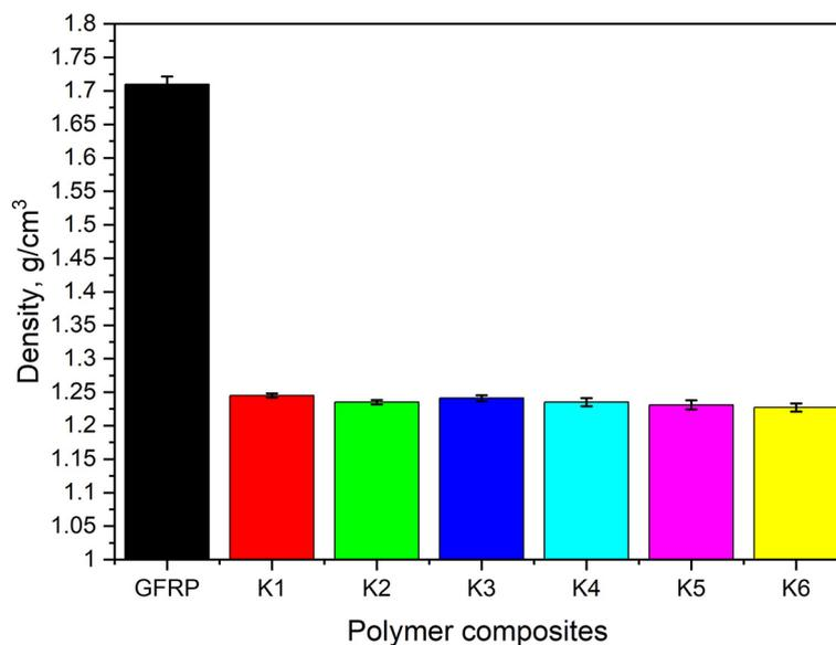
Fig. 2. Comparison of the density of HFRP (K1-K6) and GFRP composites.
