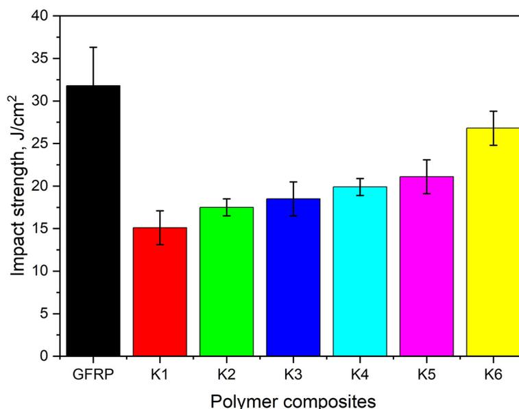
Fig. 10. Comparison of the impact strength for HFRP (K1-K6) composites and GFRP composite.
