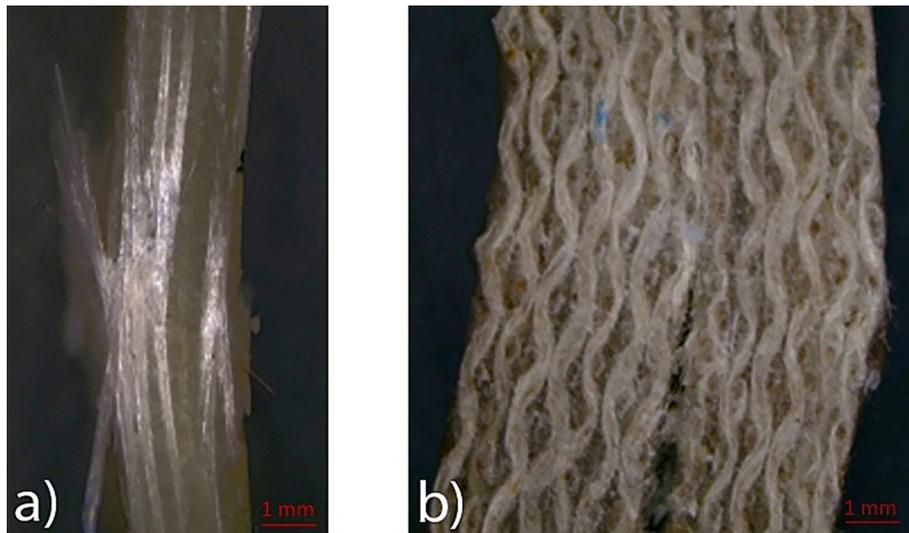
**Fig. 8.** Sample photo of the break (in a micro-scale): GFRP (a) and K6 (b) composites after the bending strength test.
