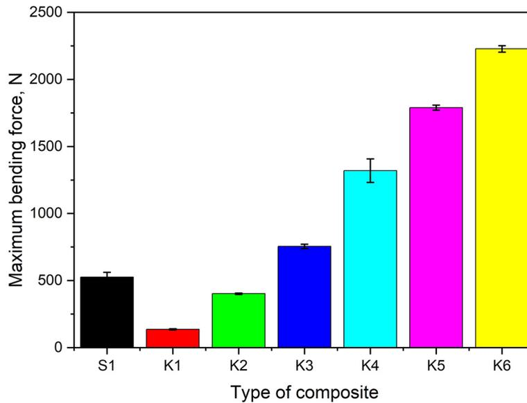
Fig. 6. Comparison of maximum bending force for HFRP (K1-K6) and GFRP composites.
