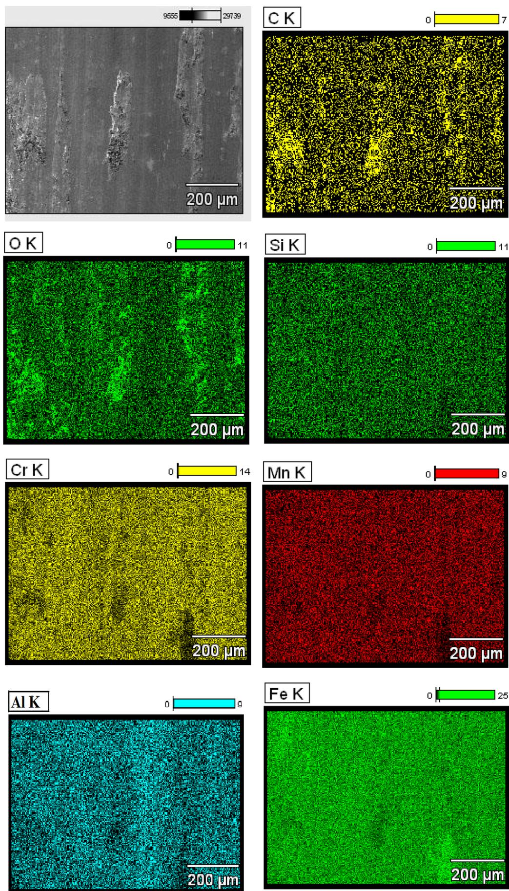
Fig. 3. Cartography of the distribution of chemical elements in the ESC from PWG
