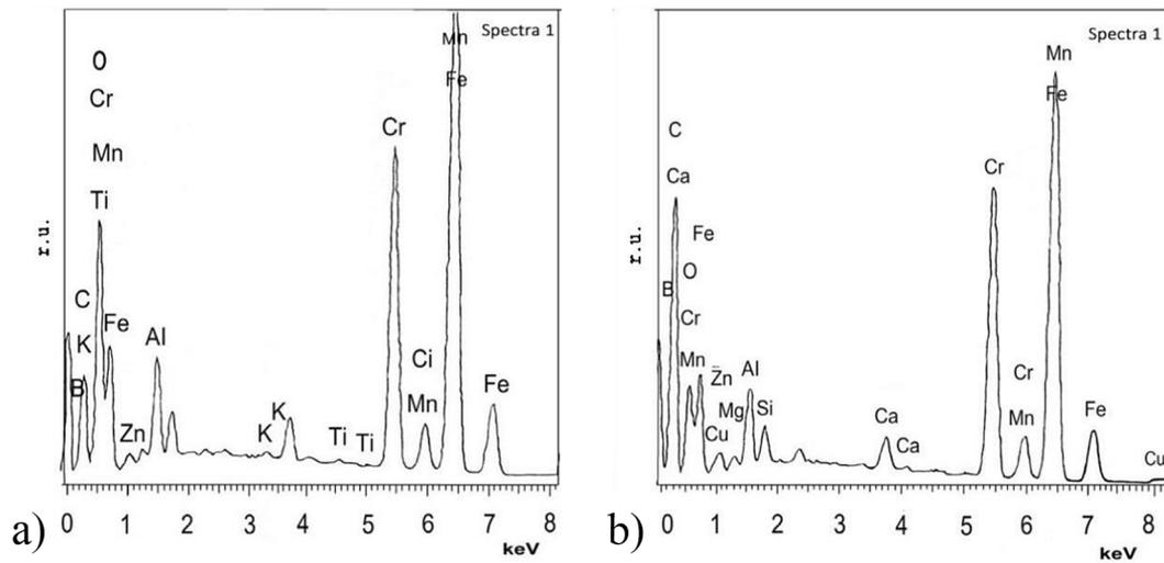
**Fig. 2.** Graphical interpretation of the chemical elements content in the ESC obtained from PW (a) and PWG (b)
