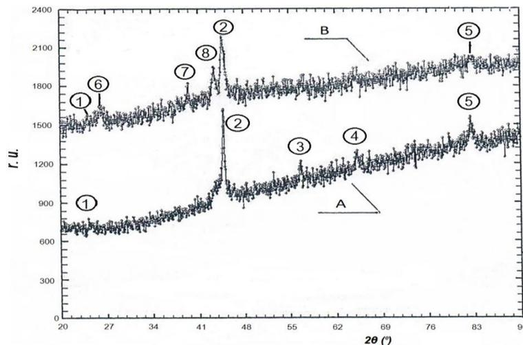
**Fig. 4.** Diffractograms of electric-spark coatings from PW (A) and PWG (B): 1 – (Fe,Cr) B; 2 – Fe (110); 3 –  $\text{Fe}_2\text{B}$ ; 4 – Fe (200); 5 – Fe (211); 6 – B (122); 7 –  $\text{Cr}_{1.65}\text{Fe}_{0.35}\text{B}_{0.96}$  (511); 8 –  $\text{Cr}_{1.65}\text{Fe}_{0.35}\text{B}_{0.96}$  (131)
