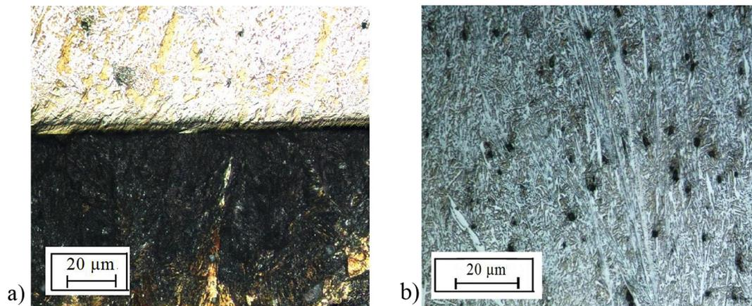
**Fig. 1.** Microstructure of electric-spark coating obtained by the PW (a) and PWG (b) electrodes, x200
