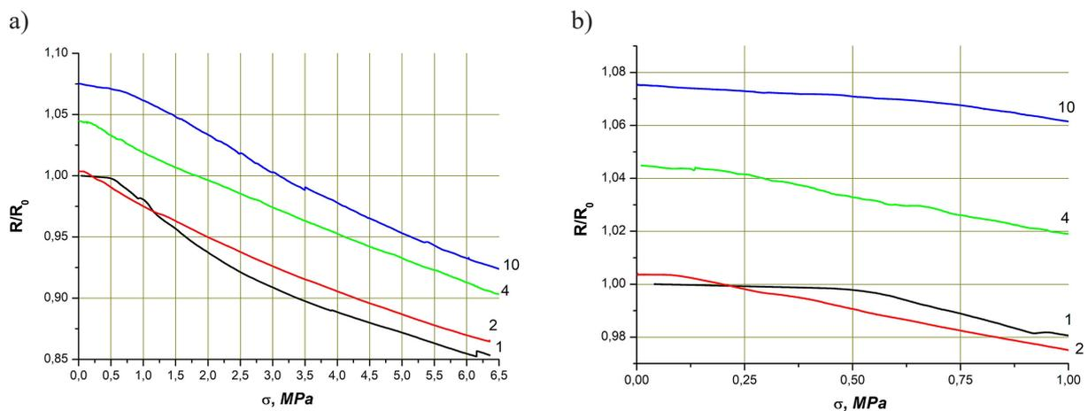
**Figure 2.** Mechano-stimulated change in the electrical conductivity of uniaxially elastically deformed crystals: 1, 2, 4, 10 – the cycles of elastic deformation (**Fig. 2b** – the initial deformation site is shown)
