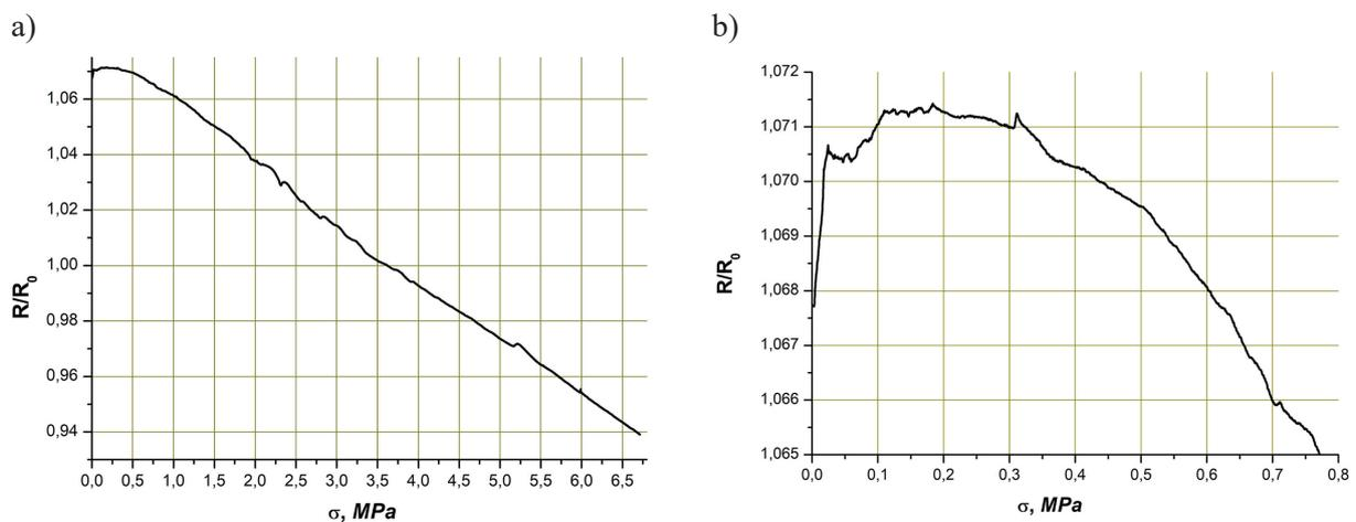
**Figure 3.** Mechanically-stimulated change in the dependence of the resistance of  $p$ -Si crystals irradiated with X-rays ( $D = 312 \text{ Gy}$ ) (in Fig. 3b – the initial section is shown)
