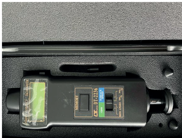
Fig. 9. Tachometer for checking the conveyors speed
