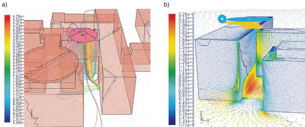
**Fig. 3.** Disturbances caused by helicopter during roof helipad operations:
