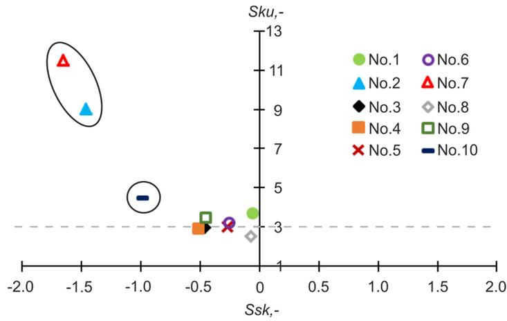
Fig. 3. The *Sku-Ssk* map of the surface for ten mixtures with metal nano oxides and graphite
