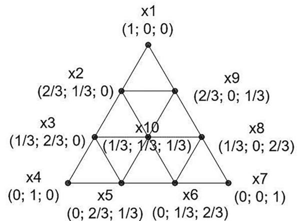
Fig. 1. Simplex lattice scheme for ten mixtures of metal nano oxides and graphite
