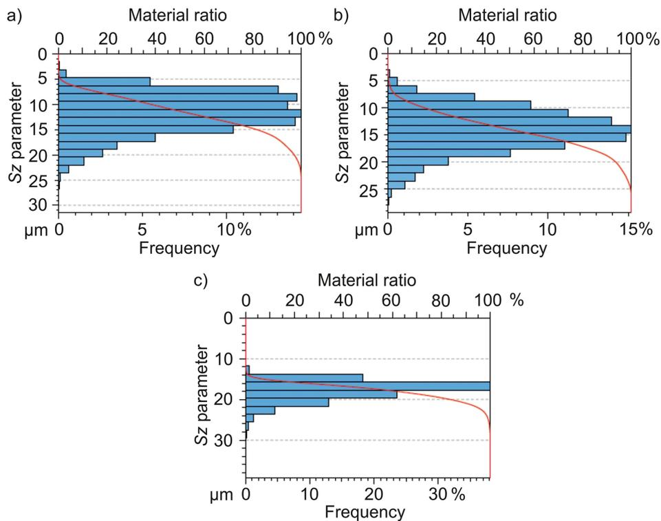
Fig. 5. Material ratio curves and peak height distribution on the surfaces after turning for mixtures: (a) Gr and  $Al_2O_3$ , (b) Gr and  $ZrO_2$ , (c) Gr,  $Al_2O_3$  and  $ZrO_2$
