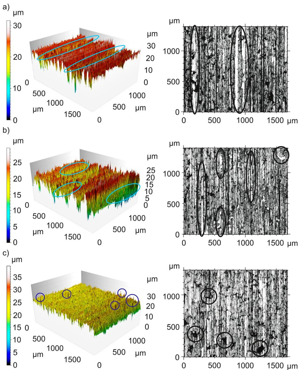
Fig. 4. 3D and 2D images of the surfaces after turning for mixtures: (a) Gr and  $\text{Al}_2\text{O}_3$ , (b) Gr and  $\text{ZrO}_2$ , (c) Gr,  $\text{Al}_2\text{O}_3$  and  $\text{ZrO}_2$ ; single defects are marked with ellipses
