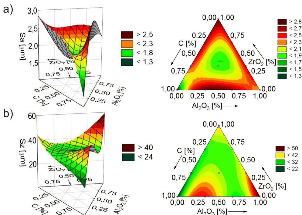
Fig. 2. Three-dimensional graphs and contour plots of changes in the amplitude parameters of the surface topography: (a)  $Sa$  and (b)  $Sz$
