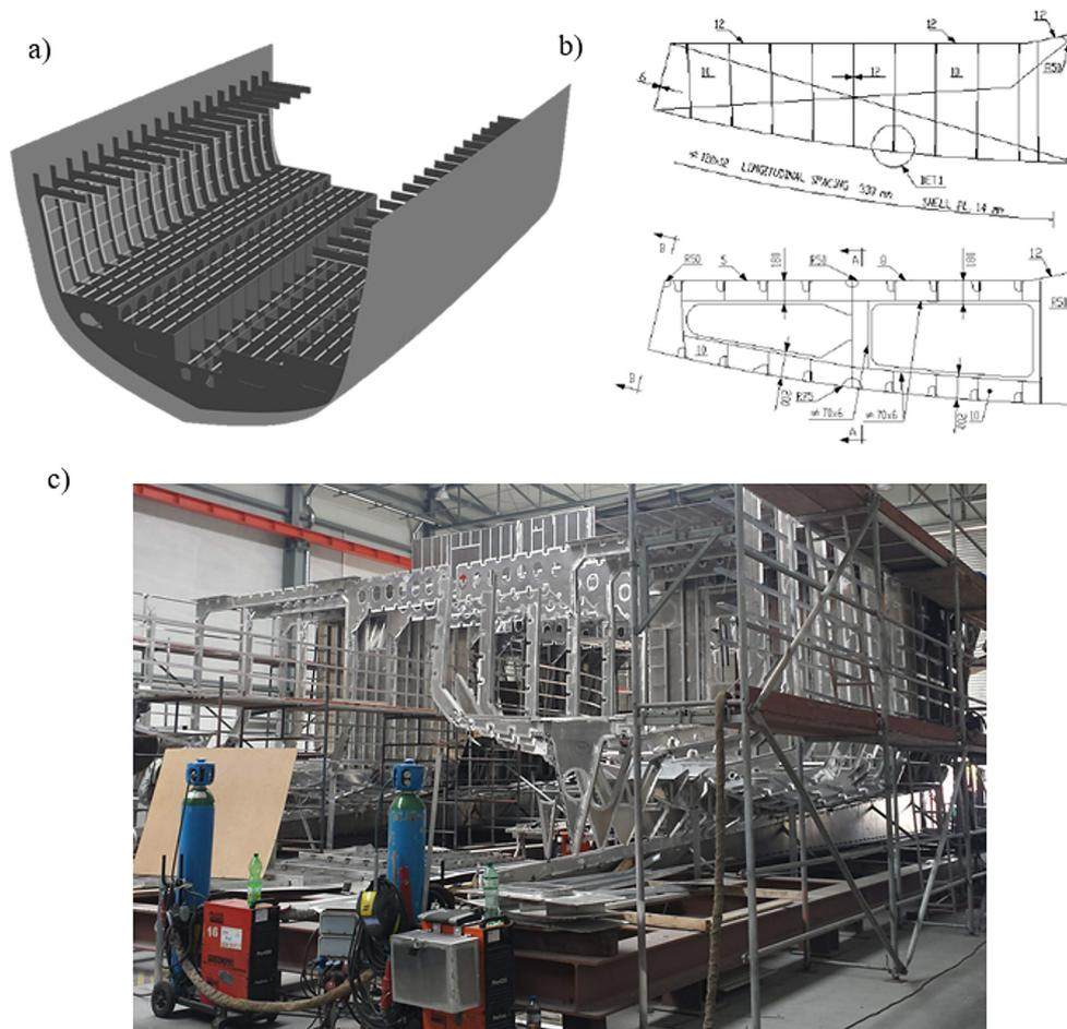
**Fig. 1.** Examples of ship structures made of aluminum alloys: a) model of yacht section – axonometric view, b) drawings of the yacht bottom structural fragments, c) frame sections in the prefabrication hall
