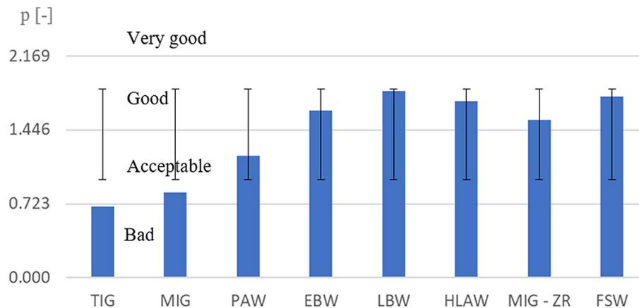
Fig. 3. Summary of field values of radar charts describing usefulness level of assessed welding processes
