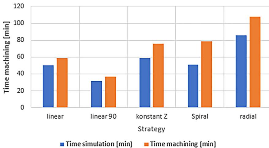
Fig. 6. Comparison between time machining and time simulation
