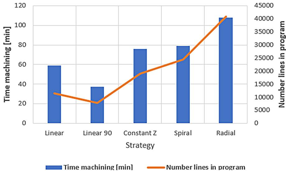
Fig. 7. Comparison of the number of lines in the program with the real machining times
