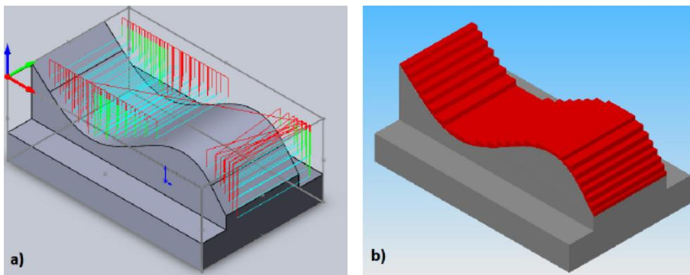
Fig. 1. Roughing operation a) tool – path of the tool b) rest material
