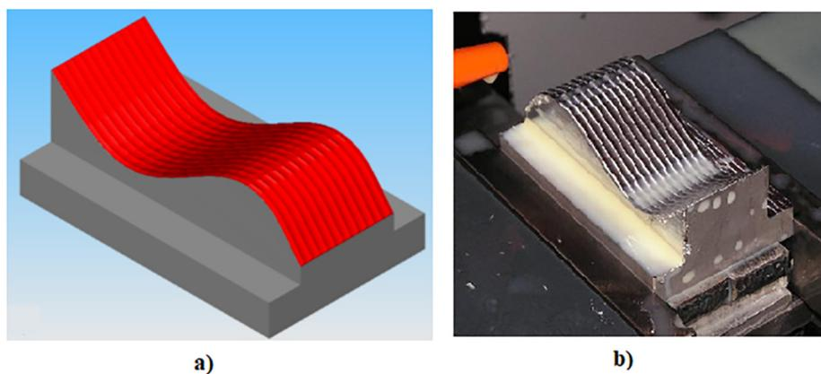
Fig. 2. Semi-finish operation a) view of rest material b) real state
