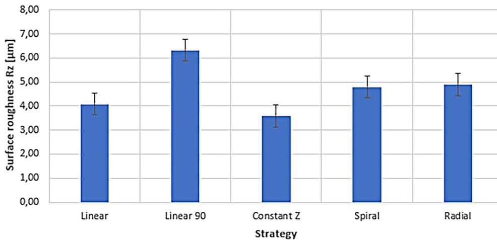
Fig. 4. The arithmetic mean surface roughness Rz comparison
