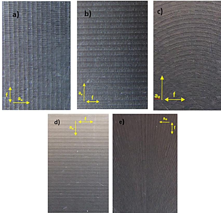
Fig. 5. Surface texture evaluation a) linear b) linear 90° c) spiral d) constant Z e) radial
