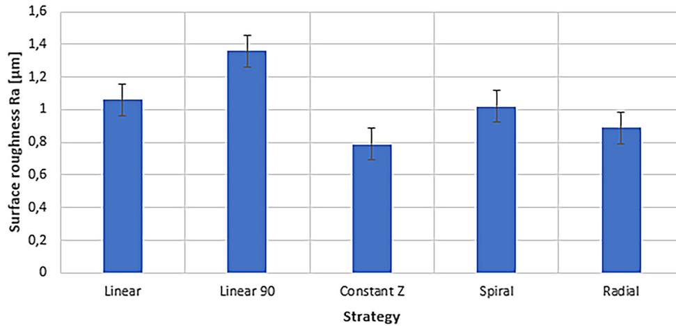
Fig. 3. The arithmetic mean surface roughness Ra comparison
