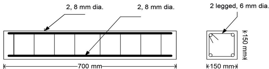
**Fig. 1.** Reinforcement detailing of beams
