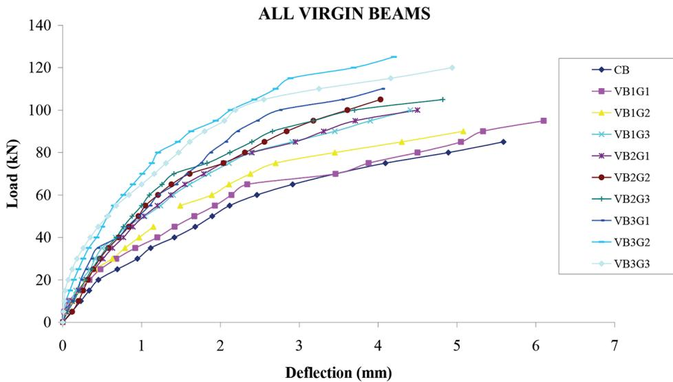
Figure 2. Load – deflection plots for CB and VB specimens
