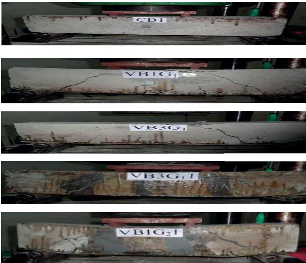
Fig. 3. Failure diagrams for beams
