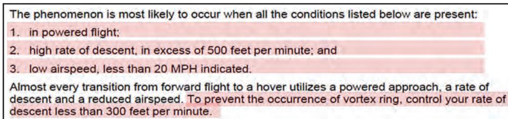
Fig. 2. The part of helicopter flight training manual about VRS [6]
