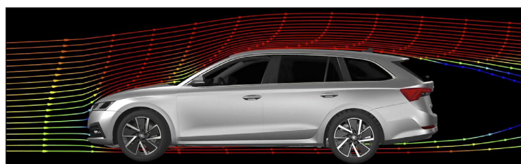
Fig. 3. Streamlines in the longitudinal midsection of a car
