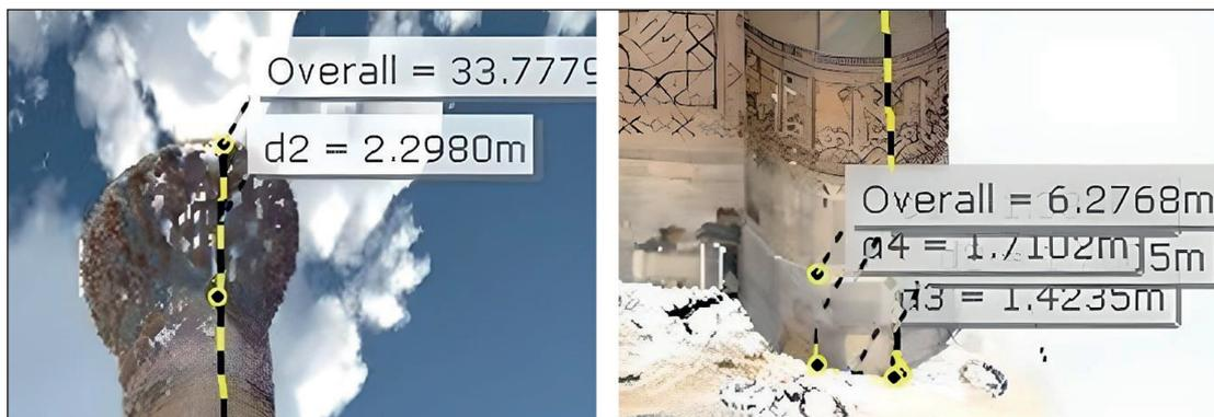
Fig. 3. 3D point cloud of the Ulugh-Begh Madrasa Minaret with marked dimensions a) head; b) base
