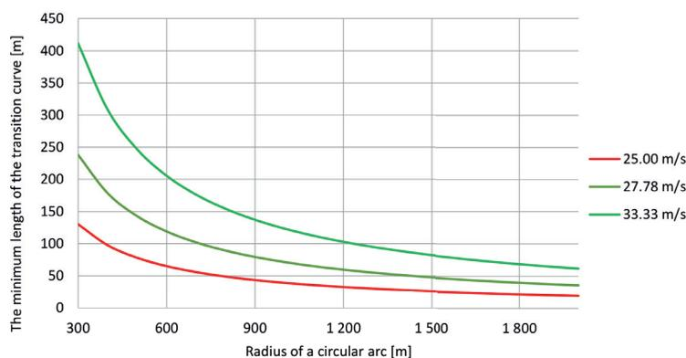
**Figure 2.** The minimum length of the transition curve depending on the radius of the circular arc for three design speeds: 25.00, 27.78 and 33.33 m/s.
