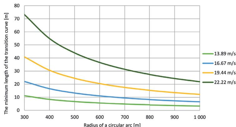
**Figure 1.** The minimum length of the transition curve depending on the radius of the circular arc for four design speeds: 13.89, 16.67, 19.44 and 22.22 m/s.
