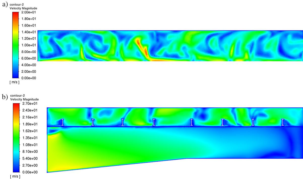
**Figure 7.** Contour velocity fields of the primary air in the control planes of the windbox of the 700 MW<sub>th</sub> Compact CFB boiler – Case C
