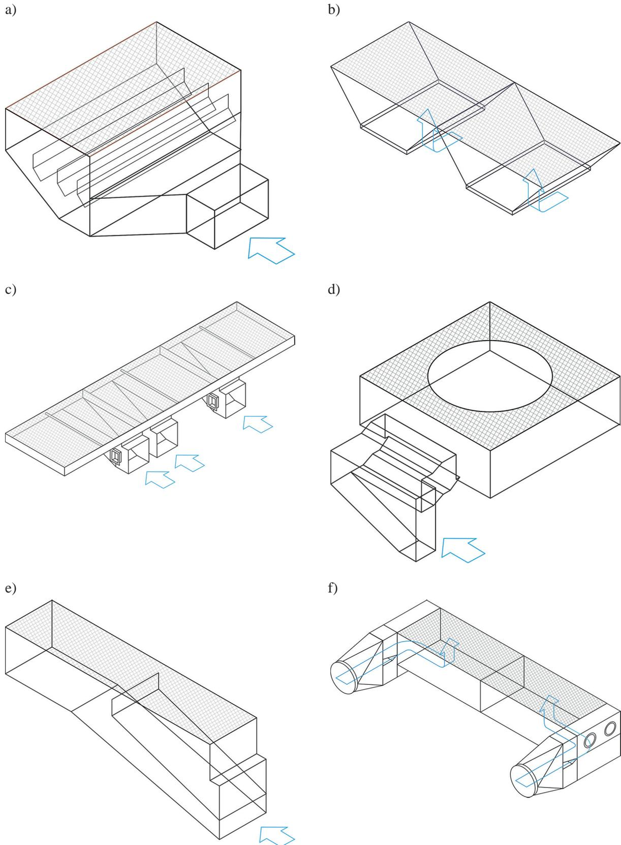
**Figure 1.** Designs of primary air plenum chambers applied in Polish CFB boilers: (a) EC Żerań SA, (b) EC Chorzów „ELCHO” Sp. z o.o., (c) PGE GiEK SA – Turow Power Plant division, (d) EC Tychy SA, (e) PGE GiEK SA – Turow Power Plant division, (f) Tauron Wytwarzanie SA – EC Katowice division [5]
