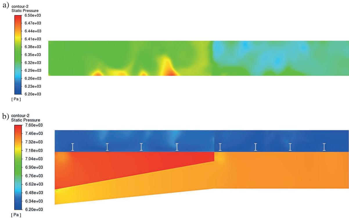
**Figure 13.** Contour static pressure fields of the primary air in the control planes of the windbox of the 700 MW<sub>th</sub> Compact CFB boiler – Case D
