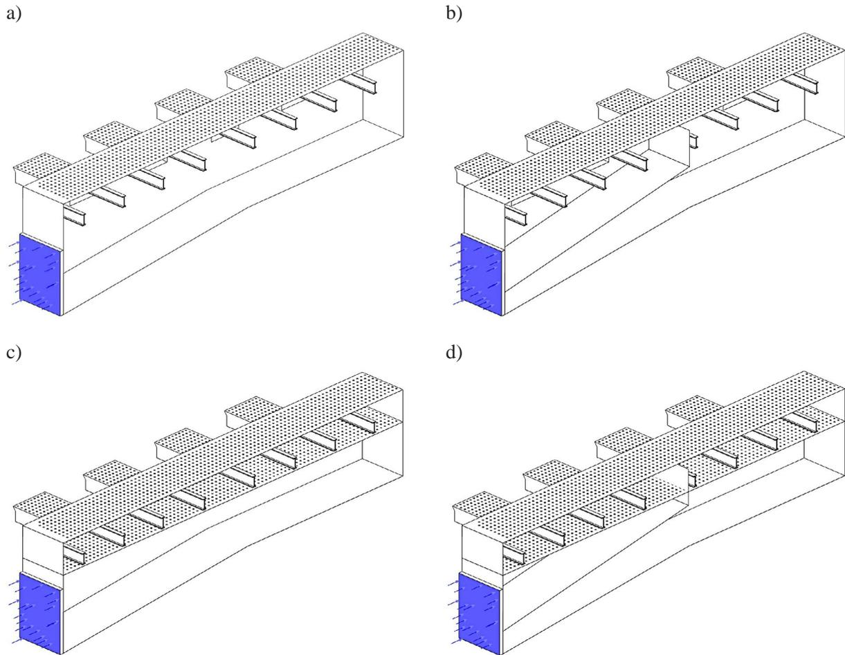
**Figure 4.** Analyzed windbox designs: (a) without the baffle dividing the gas stream at the inlet, (b) with the baffle dividing the gas stream at the inlet, (c) with a pre-distributor under the grid, (d) with the baffle dividing the gas stream at the inlet and with the pre-distributor under the grid
