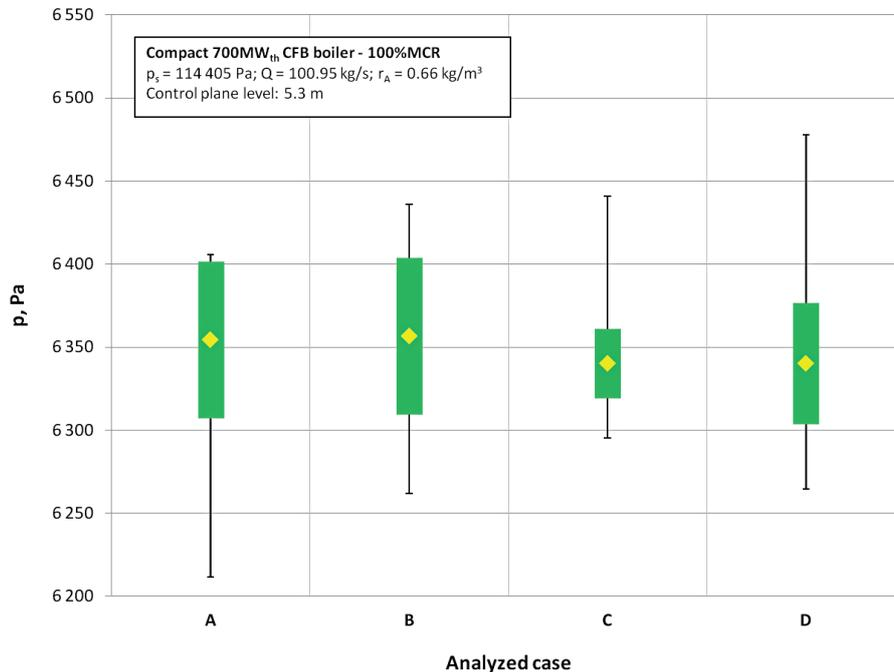
**Figure 14.** Surface integral characteristics determined for the static pressure in the control plane under the grid for all analyzed windbox designs
