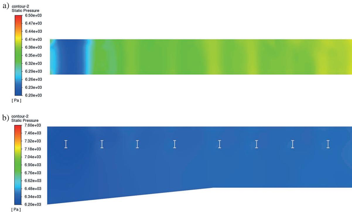
**Figure 10.** Contour static pressure fields of the primary air in the control planes of the windbox of the 700 MW<sub>th</sub> Compact CFB boiler – Case A
