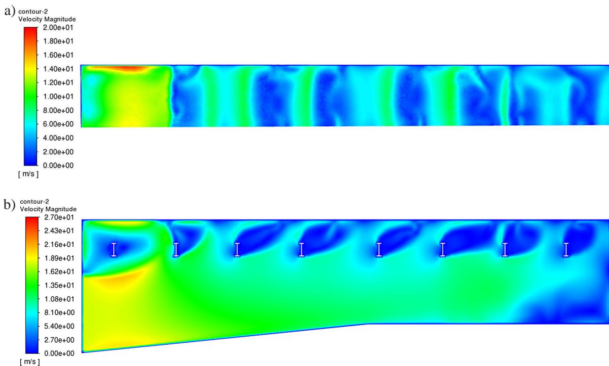
**Figure 5.** Contour velocity fields of the primary air in the control planes of the windbox of the 700 MW<sub>th</sub> Compact CFB boiler – Case A
