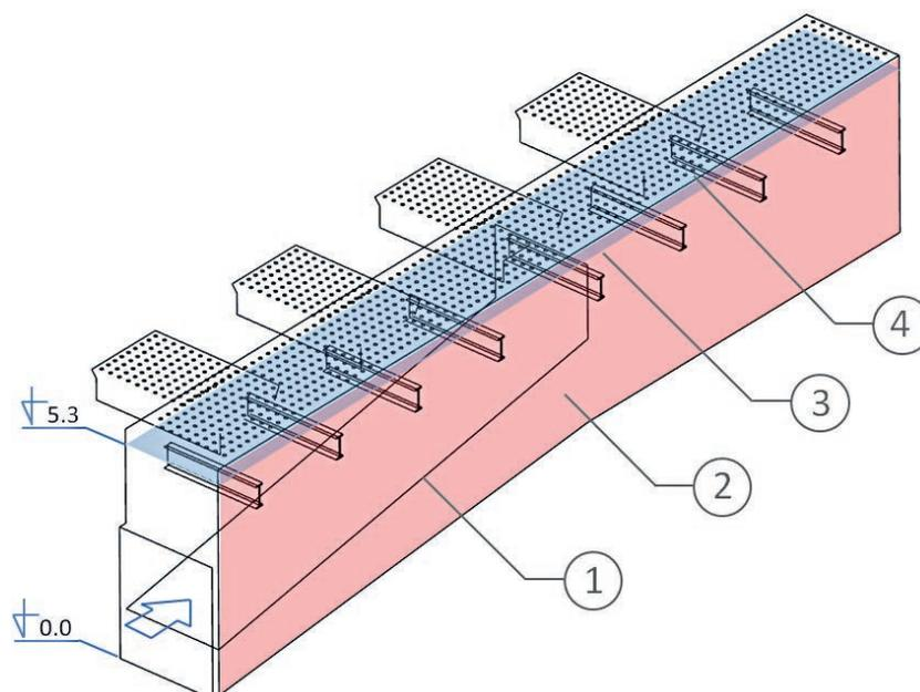
**Figure 3.** Cross-section of the 700 MW<sub>th</sub> Compact CFB boiler windbox showing the air supply cross-section, 1 – baffle dividing the primary airflow, 2 – symmetry plane (red), 3 – control plane, 4 – air distributor
