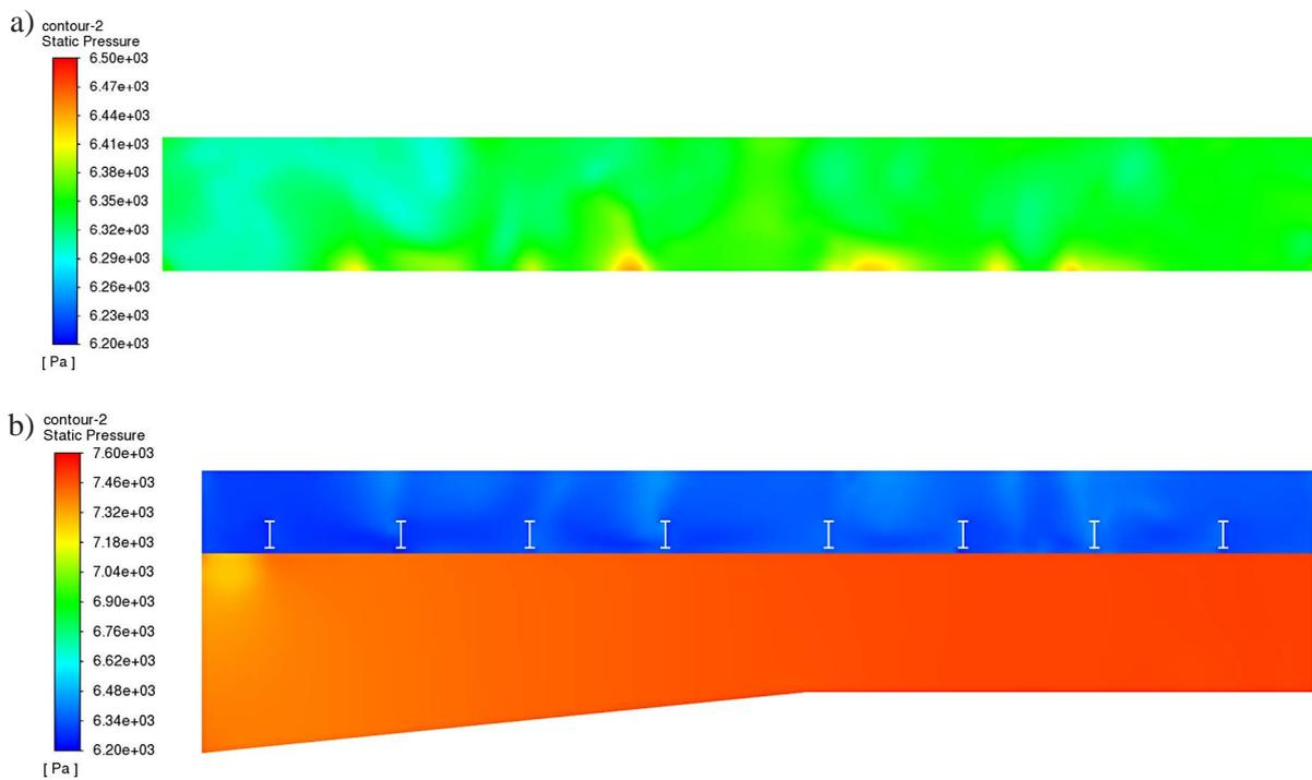
**Figure 12.** Contour static pressure fields of the primary air in the control planes of the windbox of the 700 MW<sub>th</sub> Compact CFB boiler – Case C
