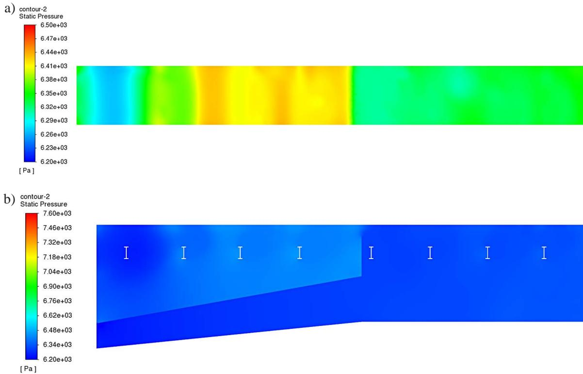
**Figure 11.** Contour static pressure fields of the primary air in the control planes of the windbox of the 700 MW<sub>th</sub> Compact CFB boiler – Case B
