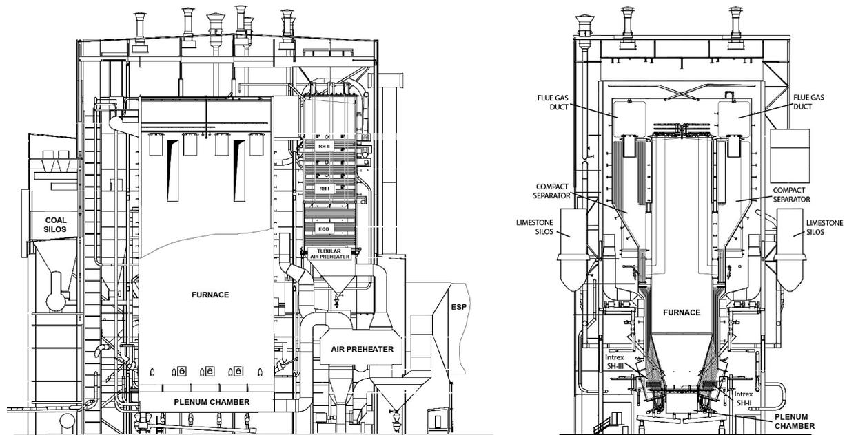
**Figure 2.** Schematic diagram of the 700 MW<sub>th</sub> Compact CFB boiler working in PGE GiEK SA – Turow Power Plant division
