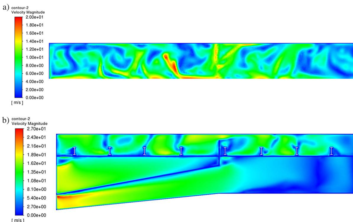
**Figure 8.** Contour velocity fields of the primary air in the control planes of the windbox of the 700 MW<sub>th</sub> Compact CFB boiler – Case D
