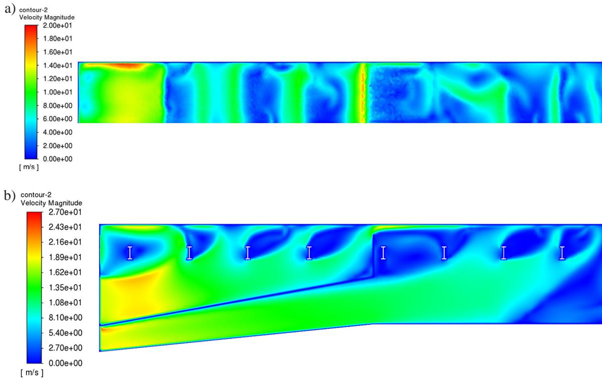
**Figure 6.** Contour velocity fields of the primary air in the control planes of the windbox of the 700 MW<sub>th</sub> Compact CFB boiler – Case B
