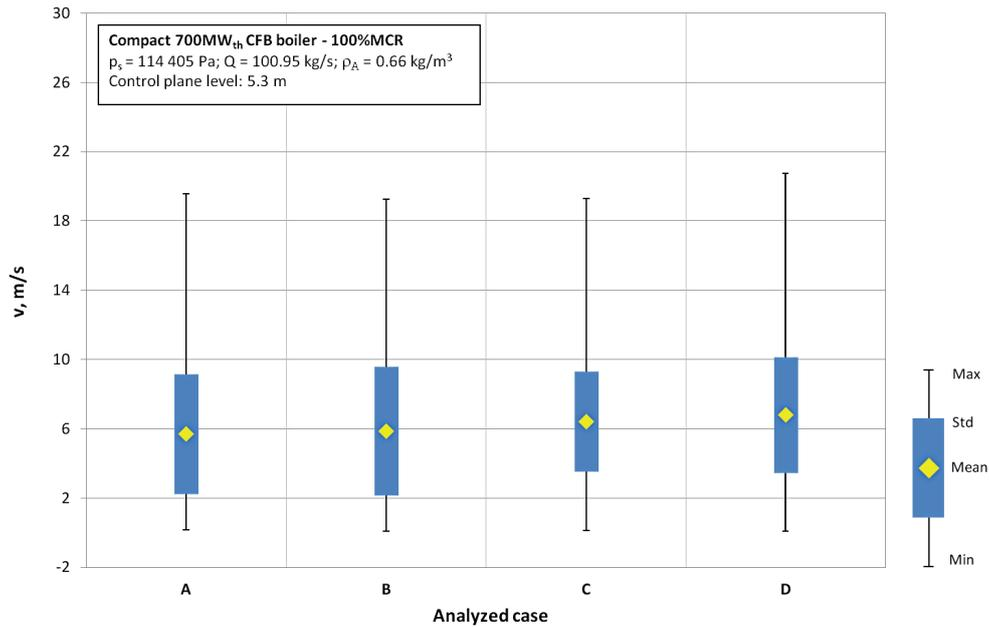
**Figure 9.** Surface integral characteristics determined for the velocity in the control plane under the grid for all analyzed windbox designs
