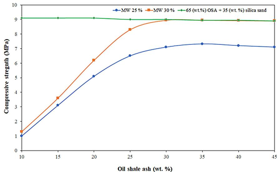
**Figure 3.** Effect of OSA content on the compressive strength of pressed specimens hardened for 28 days
