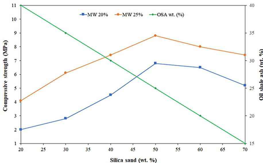
Figure 6. Influence of silica sand content on the compressive strength of pressed specimens cured for 28 days
