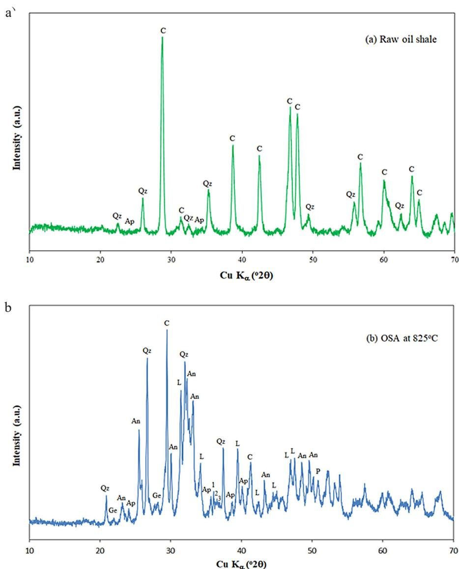
**Figure 2.** X-ray diffraction pattern of the El-Lajjun (a) raw oil shale and (b) oil shale ash. (C: calcite (CaCO<sub>3</sub>); Q: quartz (SiO<sub>2</sub>); L: lime (CaO); An: anhydrite (CaSO<sub>4</sub>); Ap: fluorapatite; P: portlandite (Ca(OH)<sub>2</sub>); G: gehlenite (Ca<sub>2</sub>Al<sub>2</sub>SiO<sub>7</sub>); 1: C<sub>2</sub>S; 2: C<sub>4</sub>AF; 3: C<sub>3</sub>A)
