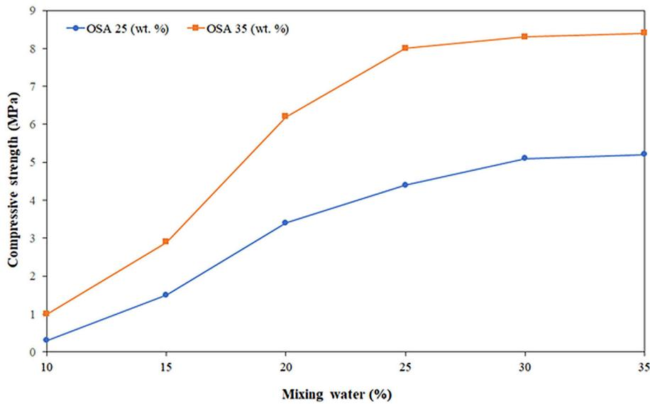
Figure 5. Effect of MW amount on the compressive strength of pressed specimens hardened for 28 days
