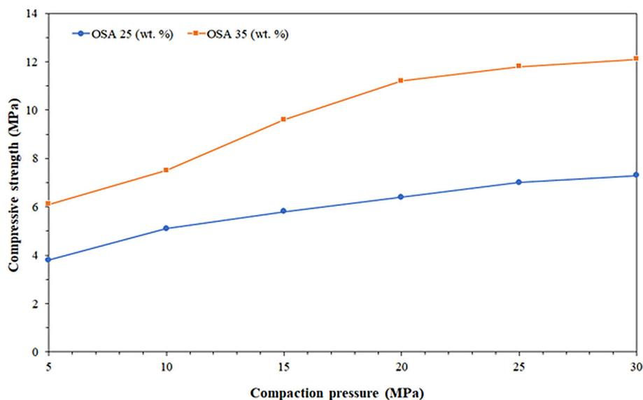
Figure 7. Effect of compaction pressure on the compressive strength of pressed specimens cured for 28 days
