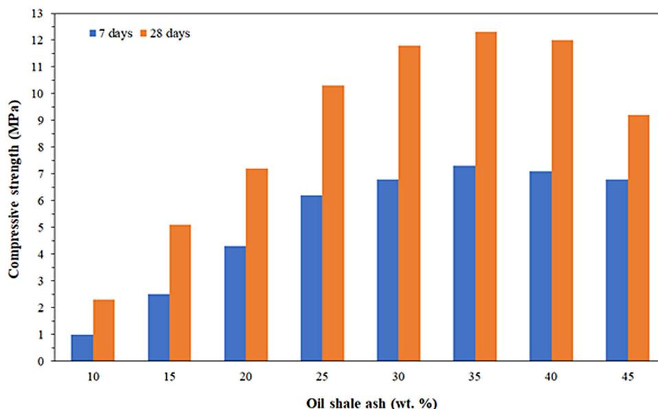
**Figure 4.** Compressive strength of pressed specimens as a function of OSA after 7 and 28 days of hardening
