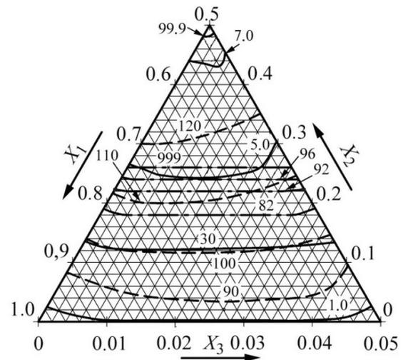
**Fig. 3.** Lines with equal composite materials property values. Solid line – adhesion strength in shear, MPa; dashed line – Vicat thermal stability, °C; dash-dotted line – content of the gel-fraction, %
