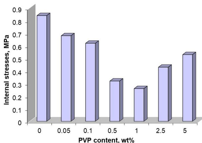
Fig. 1. Dependence of internal stresses in PFR-based glue joints on PVP content. Hardening conditions – 150–160°C for 25–30 min
