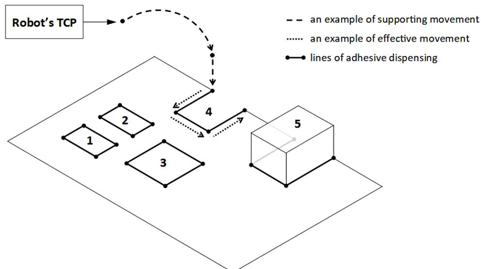
**Fig. 4.** Types of movements performed by an industrial robot in the adhesive dispensing process under analysis
