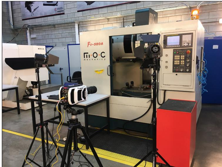
Fig. 2. Vertical machining centre FV580A with measuring equipment
