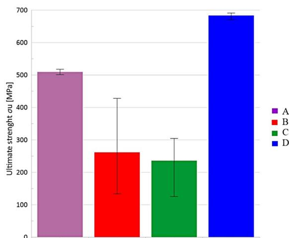
**Fig. 6.** Comparison of ultimate strength among specimen series
