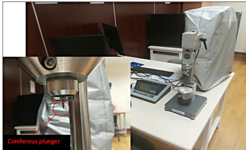
Fig. 1. Hardness-testing machine M SHORE D/C/D0 0.5 with a coniferous plunger
