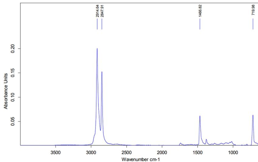
Fig. 5. ATR-FTIR HDPE spectrum of the pipe
