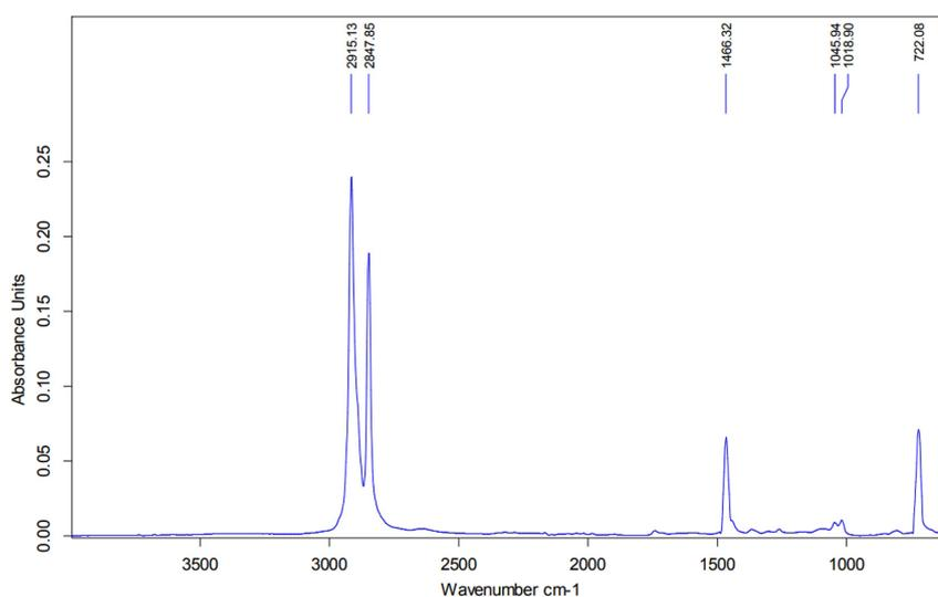
**Fig. 4.** Spectrum of ATR-FTIR HDPE Hostalen ACP 9255P
