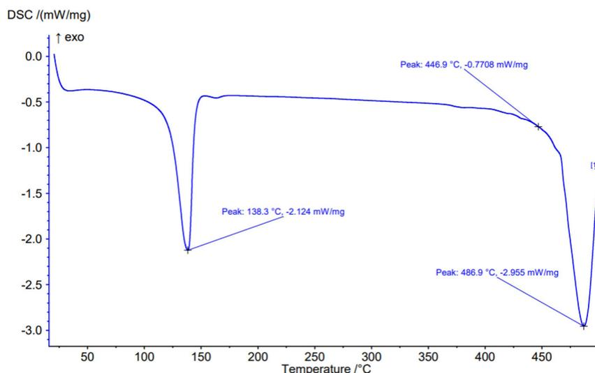
Fig. 7. DSC curve of HDPE regranulate
