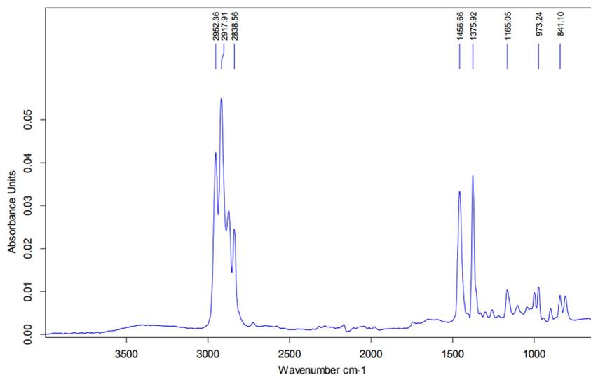
Fig. 6. ATR-FTIR spectrum of PP Moplen HP456J
