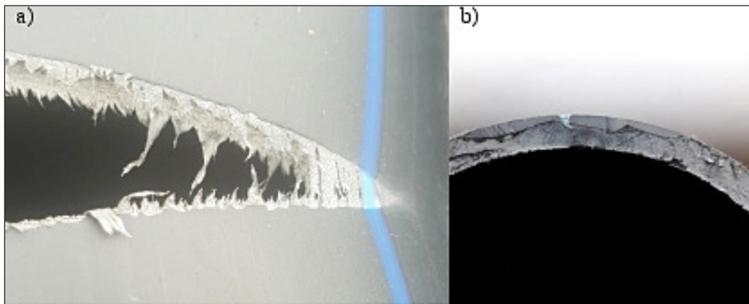
Fig 2. View of the pipe surface in the fracture area (a) and its cross-section in the beginning of the fracture's arc (b)
