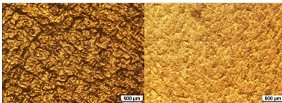
Fig. 3. Microscopic images of the recirculated (left) and fresh HDPE (right) internal pipe surface
