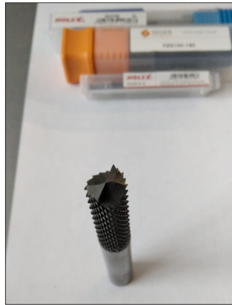
Fig. 3. The milling cutter used in the machining
