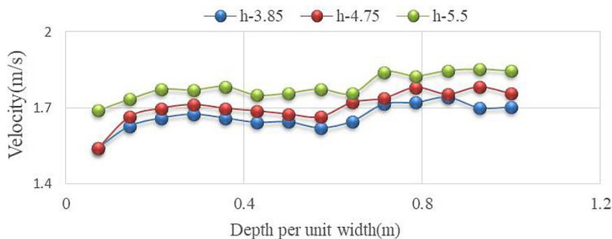
Fig. 3. Velocity distribution in section-1, rectangular channel
