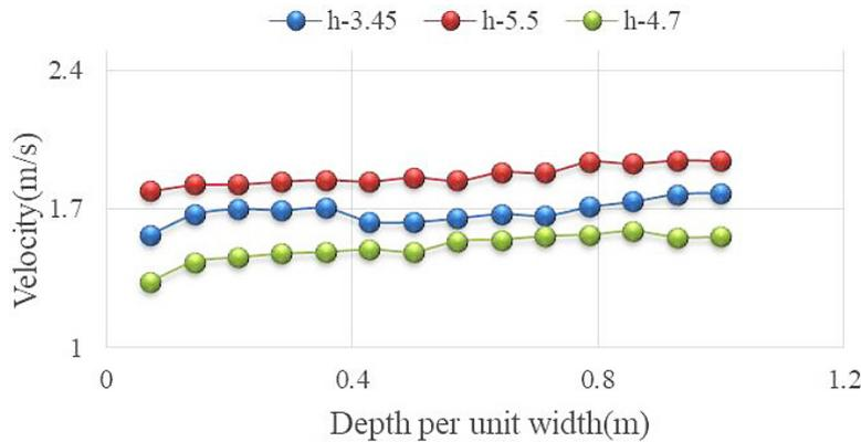
Fig. 4. Velocity distribution in section-2, rectangular channel
