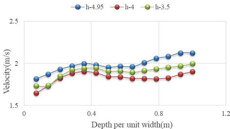
Fig. 5. Velocity distribution in section-3, rectangular channel
