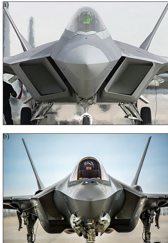
Fig. 7. Comparison of the air intake on the F-22 fighter (Fig. 7a) and its successor, the F-35 to a DSI-type design (Fig. 7b) [source : www.aviationweek.com , www.airman.dodlive.mil ]
