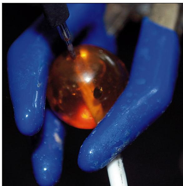
**Fig. 9.** Artificial amber after pulsed power plasma discharge in air (matte surface)
