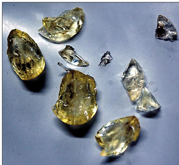
**Fig. 10.** Artificial amber after pulsed power plasma discharge in silicone oil (single shot)
