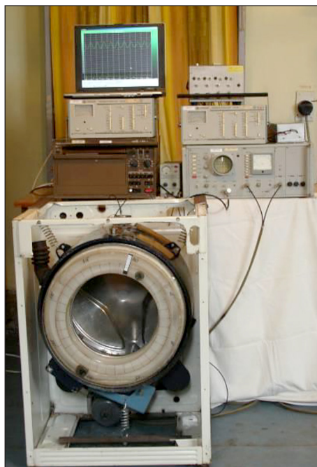
Fig. 3. General view of the experimental stand
