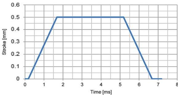
Fig. 4. Opening and closing characteristics of the injector
