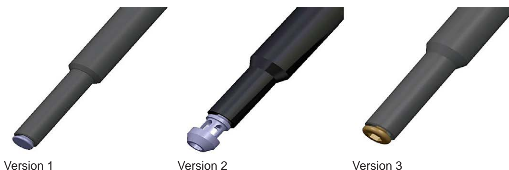
Fig. 2. Digital models of studied injectors – first from the left compatible with the real geometry
