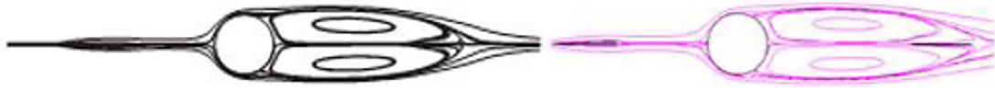
Figure 2. Comparison of streamlines in the present work (on the right) and Hwang et al. [26] (on the left). Re=100, G_1/d=1.5, G_2/d=2.4, Cd=0.91 .
