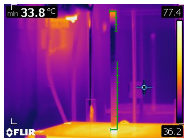
Fig. 11. ABS sample immediately after printing
