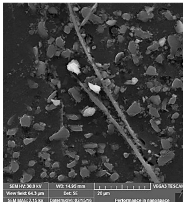
**Fig. 2.** TiO<sub>2</sub> particles distribution in PTFE matrix
