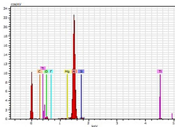
**Fig. 6.** EDS analysis – chemical composition of particles 2
