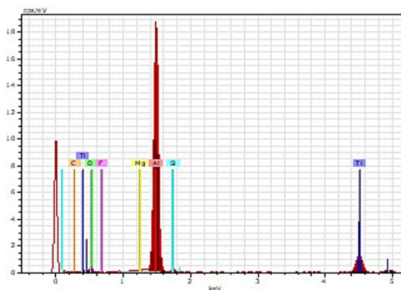
**Fig. 4.** EDS analysis – chemical composition of particles 1
