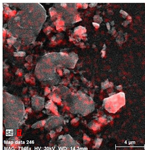
**Fig. 7.** EDS analysis – chemical element map of particles 2
