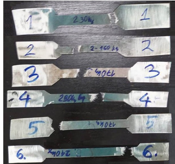
Fig. 5. Samples of elements made of glass fiber reinforced composite
