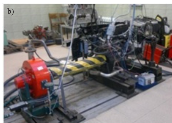
Fig. 3. a) Test bench STPiW-3 (Fuel Injection Pump and Fuel Injector Test Bench), b) Engine test bench Fiat 1,3 JTD MULTIJET 16V with dynamometer EMX 100/100
