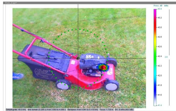
Fig. 4. The acoustic image of the dominant frequency 5000 Hz
