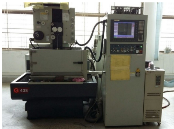
Fig. 2. Wire electric discharge machine
